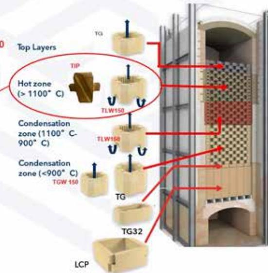
The condensation zone typically experiences the highest risk of clogging, forcing the designer to adopt shapes that reduce the turbulence of the flows. TGW shapes address this aspect, and in parallel improve the heat recovery thanks to waves on its internal surface while still mitigating blockage risks. It complements TLW by ensuring that gains in the hot zone are not lost downstream.
