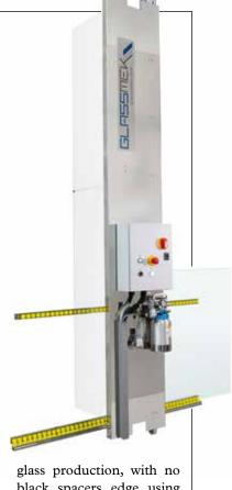
black spacers edge using transparent glass spacers and a fully automated process. Glass Company Srl developed every stage of this line internally: from glass spacers manufacturing to sealing, plasma treatment, humidity and temperature-resistant adhesives and gas filling management, including heated glass option. Full Vision IG is widely used in refrigerated display cases, internal partitions and panoramic fenestration.
