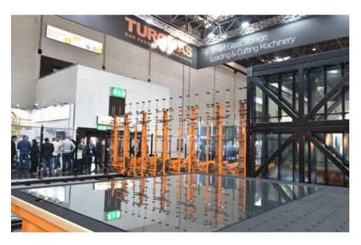
offers a cutting length of 6000 mm. The system integrates the new Turomas scoring and separation unit - reducing each cutting cycle by 10 seconds. It enables scoring with slightly heated butyral for improved quality, and the entire process
