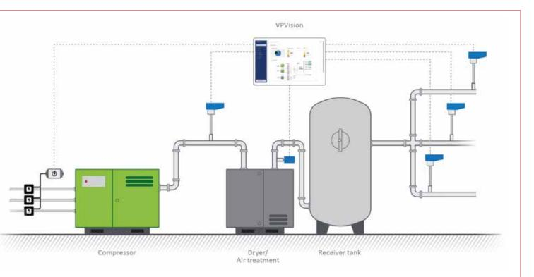
temperature and total flow at the same time, providing a complete picture. With the display, one can have a direct reading and the built-in data logger can store measurements for a longer period of time. In this way, data from the sensors can be analyzed and action taken, if necessary. VPVision even provides real-time insight into energy flows, wherever the user may be.
