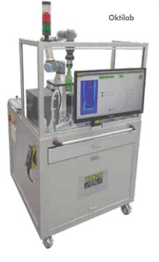
**Strain View** is Tecnosens' solution for the automatic monitoring of residual stress in glass containers. The system performs accurate and repeatable measurements on both the bottom and side surfaces, ensuring compliance with quality standards and helping to prevent breakage, contamination, and non-conformities.
