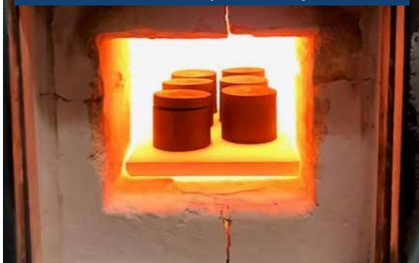
Graphite crucibles are needed to form the pucks used for XRF compositional analysis
