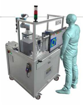
meet growing demands for automation, accuracy and ease of use. The system can automatically inspect a wide range of characteristics in glass containers, including:
