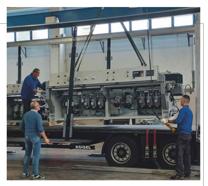
extraordinary working speed that reaches 10 metres per minute. It capably manages glass thicknesses from 3 to 55 millimetres with an installed power of 22.7 KW. The conveyor system with rubber pads on steel guides doesn't need continuous lubrication, while the touchscreen PLC allows the total control of all the parameters and troubleshooting. Need more data? Minimum dimensions: 100x100 mm Max. load: 1800 kg Height of working surface: 840 cm
