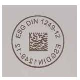
When the glass ID is included in the code, the number can be read by a scanner or mobile device.
