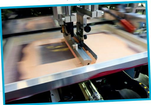
using thermoplastic inks and up to nine in the case of UVLED inks. Here the ability to print up to ten colours inline allows the creation of complex, highdensity graphics - expanding opportunities for both packaging customization and aesthetic enhancement.
