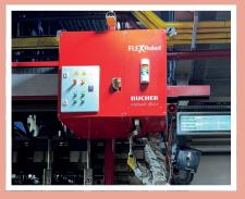
and 1.15 kVA in standby mode. Compressed air requirements include a pressure of 5 bar and a flow rate of 1000 liters per minute. The recommended operating temperature ranges from 0 to 45°C - ensuring reliable functionality within a broad industrial environment.
