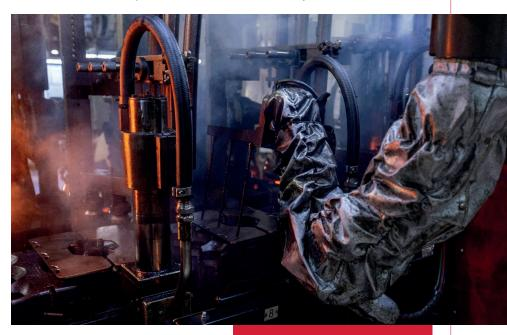
During an 8-hour shift on a 36-cavity machine, an operator performs over 1700 swab movements and lifts the arm to activate the manual swab cycle more than 550 times. Using a FlexRobot Blankside eliminates strain injuries caused by repetitive manual swabbing.
