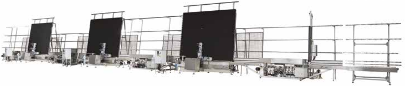
Automatic straight edging line mod. TURNOVER
