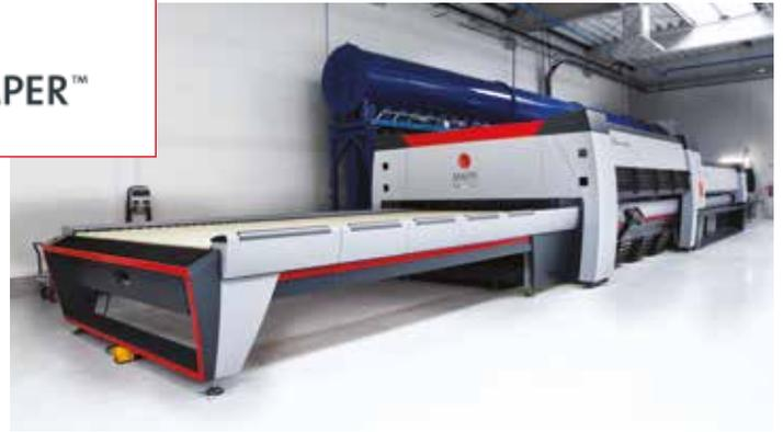
**ESS | ENERGY SAVING SYSTEM** Heating and forced ventilation stages are coordinated and managed by a computerized system optimizing consumption and significantly reducing the installed power required by the entire system.
