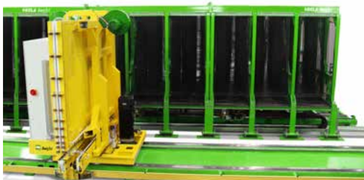
HEGLA SortJet: Invented to reduce material costs and improve production flow
