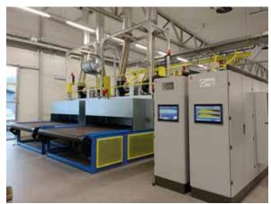
design. The burners installed on the lehrs are patented by CAR-MET, adapted to almost any type of gas. Size and configuration of each lehr is based on the space available for the installation and type of production. Heating and cooling systems installed have been developed in accordance with European energysaving regulations; which reduce operating costs in energy consumptions.
