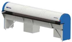
**AGIL TR** is a super compact, versatile and easy to install cutting table. It automatically cuts float glass sheets and semi-automatically cuts laminated glass sheets, thanks to the double-zero system. Agil tr can process sheets up to 3810x2600 mm, has 4
