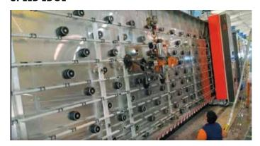
BSolution's Speed Edge is a vertical compact grinder with the innovative patented follow-glass system, which carries out both rough and polished machining, flat and round edging, arising and milling.
