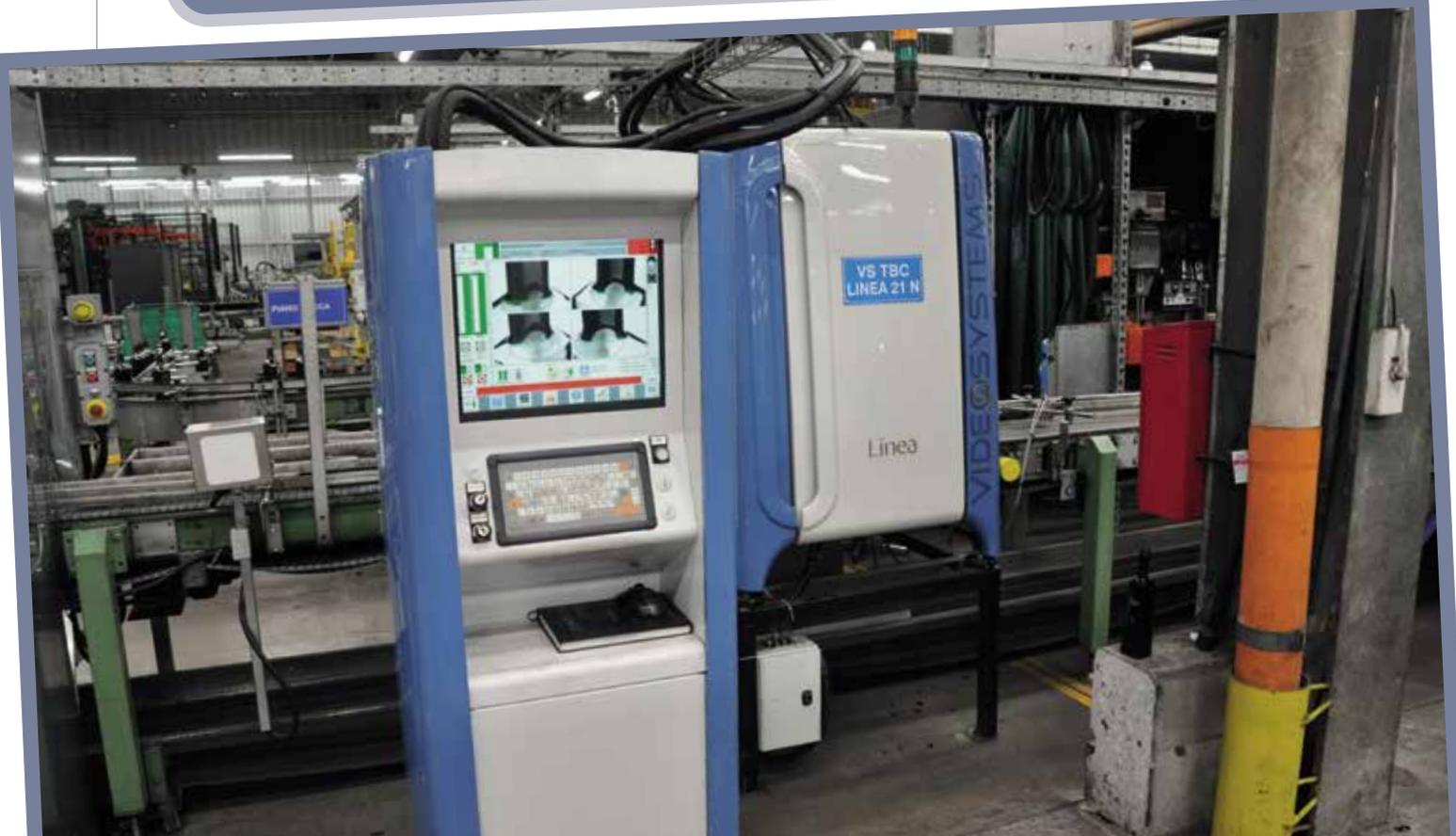
**G**lass container inspection processes have been characterized for decades by human manpower and optical inspection technology. The ability to identify many types of defects has increased thanks to innovations on electronic and optical devices, but some types have no real solution.
