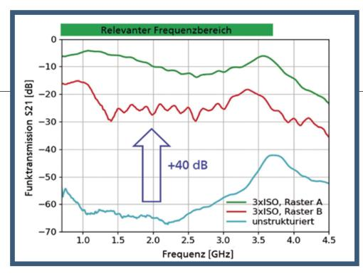
GHz need segments that are much smaller than 8.8 cm ( $\lambda/4 = 2.2$  cm). But heat protection also needs to be retained at the same time. Different segment geometries demonstrated a significant improvement in the frequency ranges relevant today. Nevertheless, radio wave transmission cannot be increased equally across all frequency ranges, as one grid size remains always fixed.
