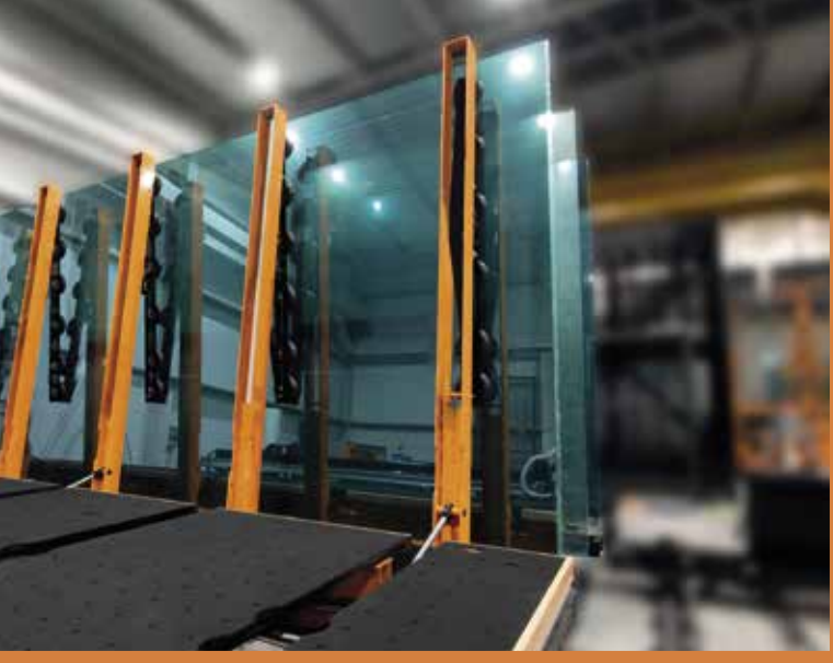
New TUROMAS loading system integrated in the RUBI 406VA cutting table
