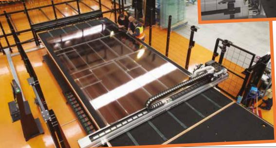
table. To ensure the linearity of the hose, as well as correct air flow, it's guided by cable chains specially-designed for the function.
