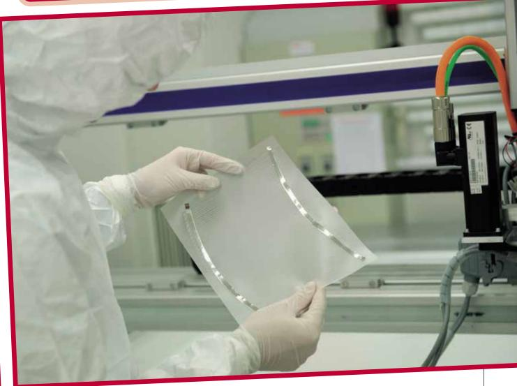
with heating wires" for glass factories worldwide, also applying special "wire antennas in windshields" in high quantities following the latest trend among car manufacturers.
