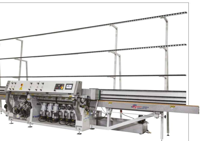
the presence of glass, then measure its thickness. They stops the glass sheet so that to give time to set the conveyor and release it. Here, in the interests of compliance, sheets will typically continue to be processed. However, should the sensors detect some discrepancy, the machine will independently ensure that the conveyor becomes conformant with the thickness detected - thereby adjusting the processing speed based upon previously set parameters.
