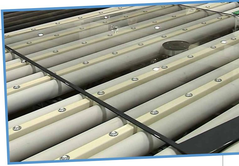
LASSLINE is Rollmac's machine made to varnish the four edges of flat glass sheets by means of a steel engraved cylinder, both with ceramic glazes or cold varnish: it responds to the demands of construction and furniture companies that need specific processing techniques on the edges of glass flat sheets.
