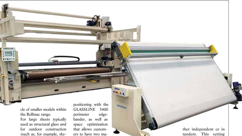
(such as, for example, skyscraper wall cladding), the new solution by Rollmac, a division of GEMATA Spa, works with an engraved roller in reverse mode and has a maximum working width of 3300 mm and a sheet thickness from 2 to 19 mm. Coating quantity can be set from 50 g/m<sup>2</sup> to 350 g/m<sup>2</sup> (i.e. from 30 up to 220 microns) in a
