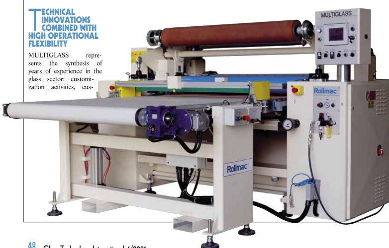
A machine that combines the latest technical innovations with high operational flexibility. This is the description of MULTIGLASS, Rollmac's machine for enamelling, painting and design printing operations of small and large float glass sheets.
