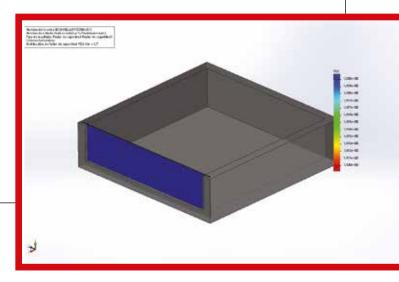
ing analysis of each layer comprising the final glass, thicknesses that meet the requirements established by the client are verified - providing an optimum solution for their application. In short, it is about guaranteeing project safety with a correct dimensioning of the glass thicknesses that will allow an optimal cost-safety ratio.
