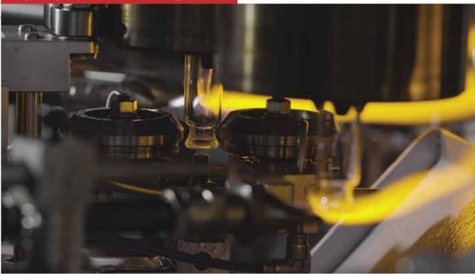
The machine has been developed to reach a maximum output of 55 pcs/min. with 2R vials, with the possibility of processing glass tube diameters from 10mm to 30mm.
