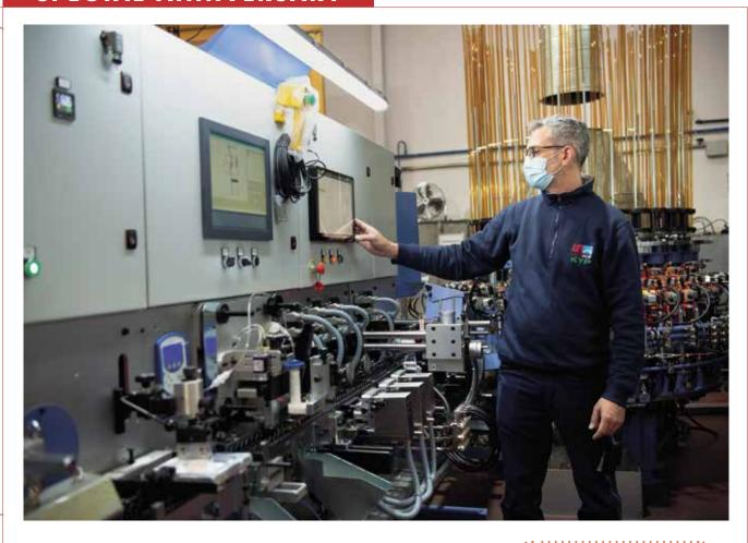
From the machine control panel, the operator can easily set the starting and ending positions of the plates and cams driven by servo-motors via user-friendly software. During setting and job-change operations, the operator can use remote push-button by enabling the jog mode.
