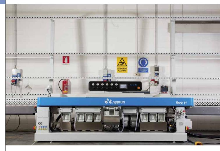
within the Rock series feature the patented conveyor in double material. The shell is made of highly mechanically resistant material that's especially designed to grant structural rigidity. Furthermore, the part in contact with the guides is made of wear-resistant, long-lasting Kevlar. This solution is a new milestone in conveyor durability, guaranteeing a working life that extends to more than 2 million linear metres.
