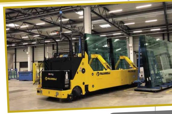
with jumbo or LES glass. Not only. The transporter slows down automatically whilst loading, thereby stopping to avoid hitting the rack at loading.
