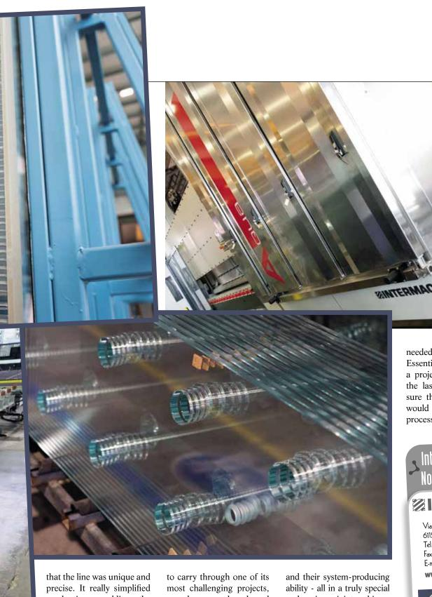
precise. It really simplified production, enabling the glass to be ground, bored and tempered within the integrated line created, and without any sheet unloading and reloading." Indeed it's thanks to this system that Novavetro's been able
