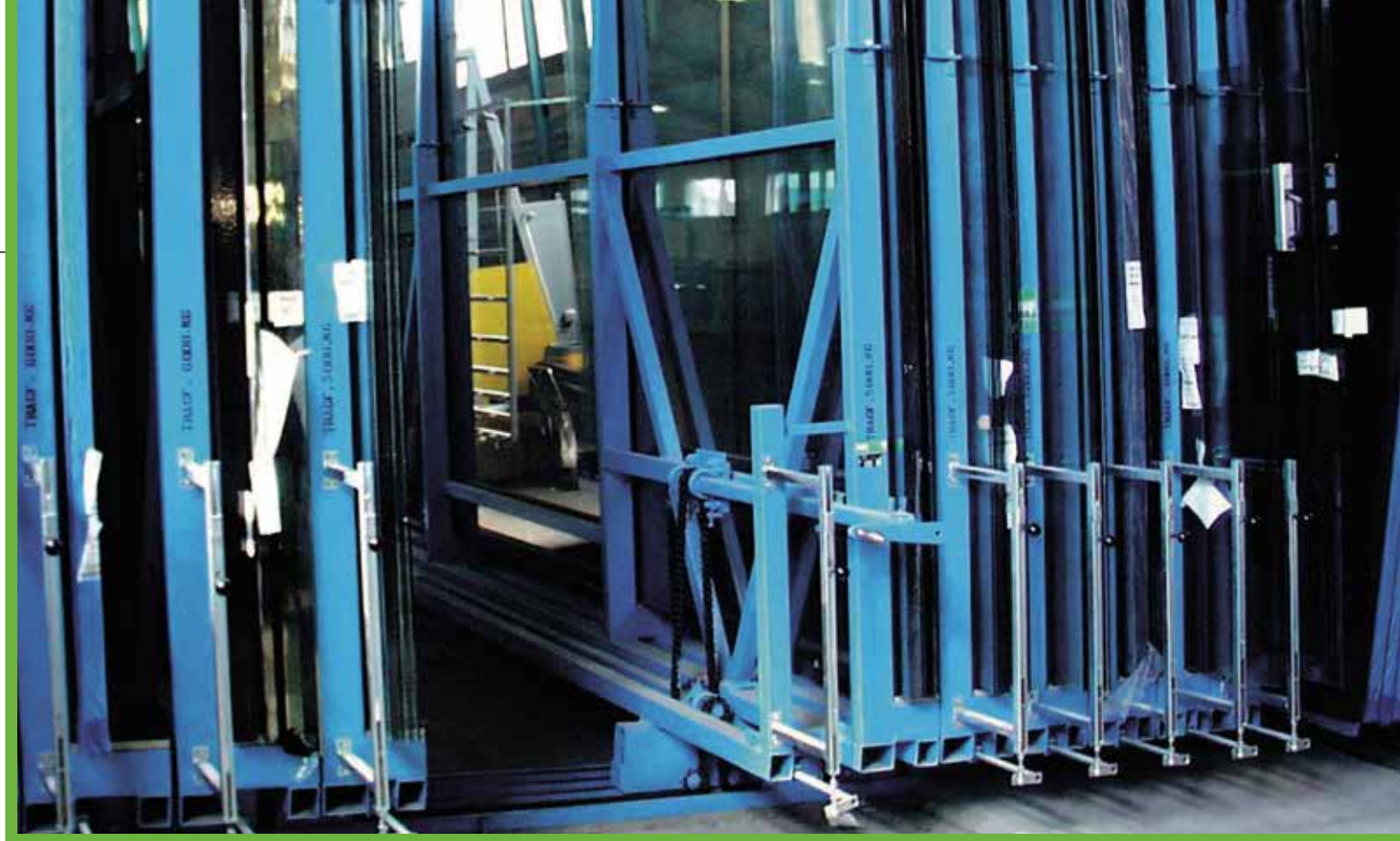
Manual compact storage system for glass. Operators can easily move individual storage racks as they are on a special track system
