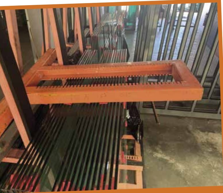
Glass to be placed through the back of the A frame once the pole has been released.
