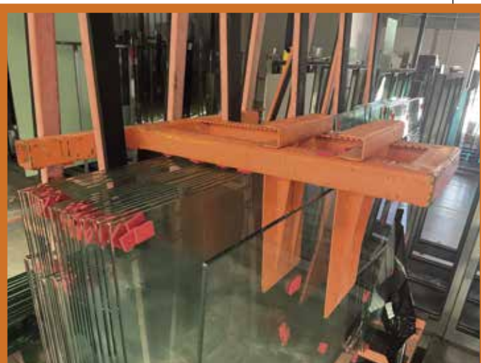
Lean a single piece out against the remaining paddle. This creates space to place the free paddle back in, tight against the remaining glass. The glass is kept in place whilst the front piece is removed.
