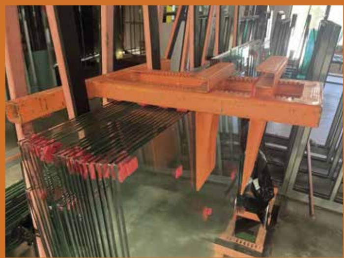
Outer paddle to be moved and placed further away from the inner paddle.
