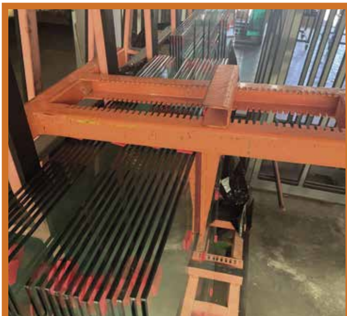
Inner paddle to be inserted closest to the glass to keep it in place.
