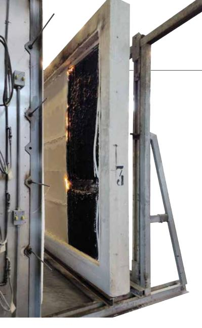
the ability of an element to resist any passage of flames and hot gases to the side unexposed to fire, (W) indicates radiation resistance, i.e. the ability of an element to resist fire acting upon one side only, thereby limiting heat transmission by radiation to a specific threshold, (I) indicates isolation, i.e. the ability of an element to withstand exposure to a fire acting upon one side only, thus preventing it from spreading.
