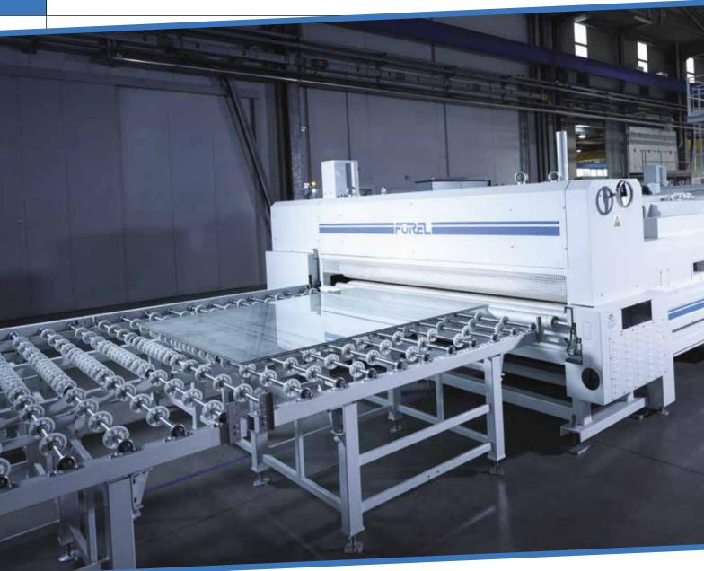
apable of flexible production with its PVB and SentryGlas® interlayer, Forel's latest Art. LL lamination line for producing laminated glass comes as an optimum solution for the processing of different sizes, shapes and types of glass.
