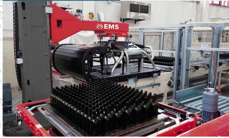
separator (flap/tray/cap) on each layer. This cycle is repeated by the palletizer until the expected number of layers has been transferred to the pallet.
