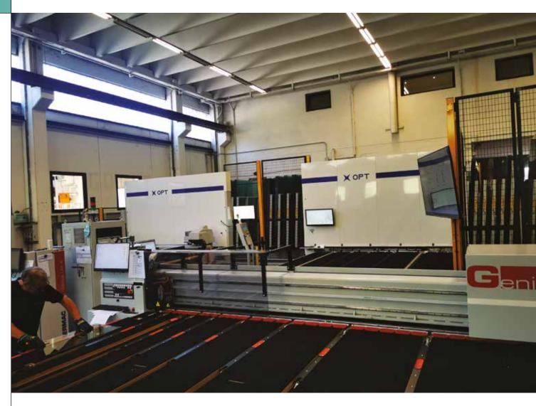
ble - essentially detecting non-conformities and evaluating them on the basis of user-defined parameters. In this way a defect map is created which is then sent to the cutting table to be either shown to the operator or used for automatic re-optimisation of the cutting plan.
