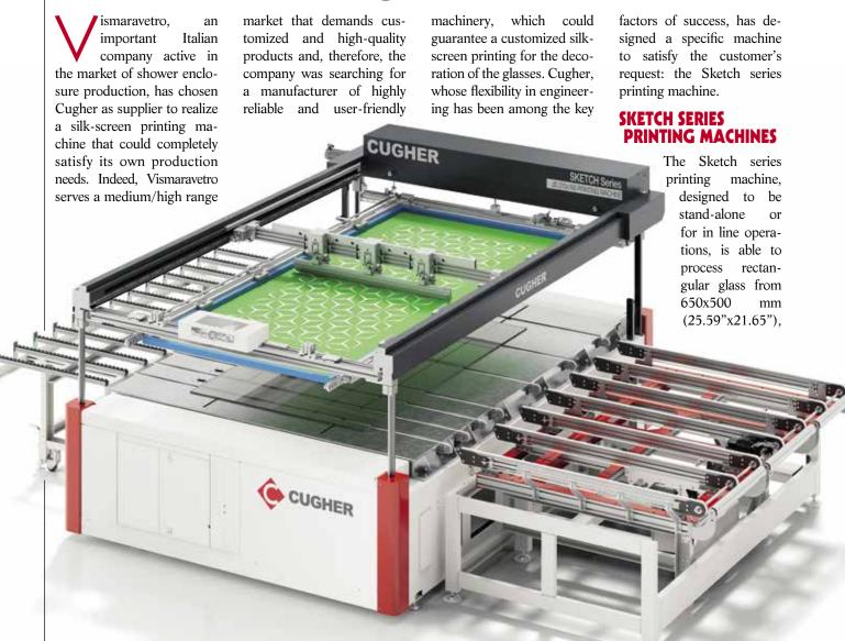
Silk-screen printing, consolidated technology for which Cugher provides high performing machinery, guarantees excellent image definition, the uniformity of the ink over the entire surface of the glass and high coverage. These are the characteristics required by glass manufactures that provide solutions for the interior design sector, such as decorations for shower enclosures.
