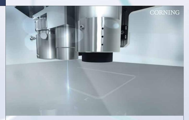
ting of the most complex and demanding geometries and improved edge quality. Higher edge strength, lesser need for post-processing and improved break resistance are further benefits enabled by Corning's Enhanced nanoPerforation process.
