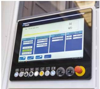
the machine automatically measures the incoming glass (height, length, and thickness) and processes the edge. Not only. CMS Aura will also adapt its operator units to different thicknesses.
