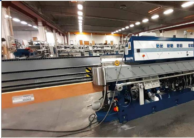
sponds to the needs of the reference markets – architecture, interior design, home appliance – combined with the technological push that the company puts in all its products, together with its subsidiary Bovone Diamond Tools. The in-depth study of tools has led the company to use and configure the grinding wheels in such a way as to allow to create a stair groove and arris in a single step.
