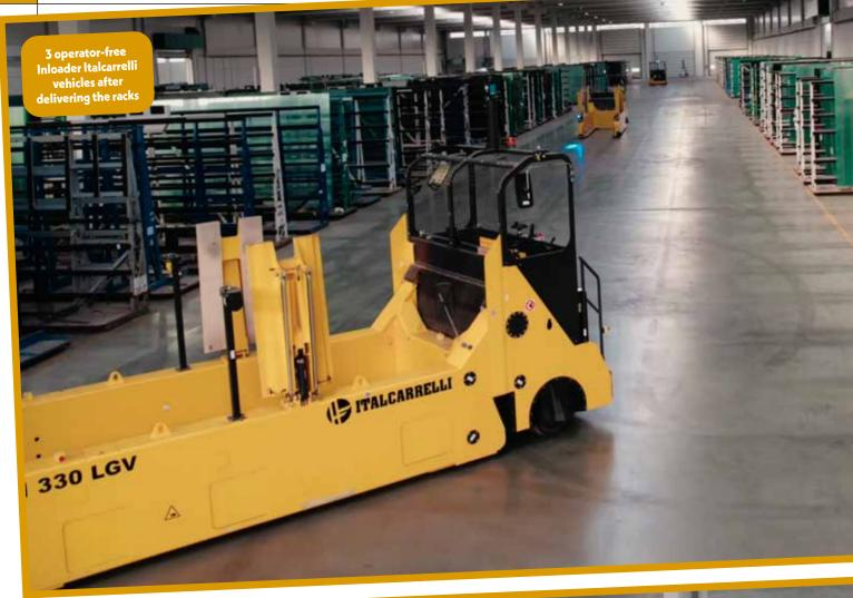
threshold, the vehicles proceed to the charging area, where automated battery swapping occurs. This process ensures uninterrupted operation - so avoiding downtime caused by charging and ensuring consistent productivity.
