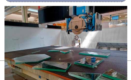
3000 mm/min, the ability to process glass with thicknesses up to 100 mm (depending on the cutting disc), and a 33 percent increase in productivity thanks to the onboard manipulator. These features make the CMS Sprint the ideal solution for fire-resistant and safety glass cutting, providing superior performance and operational efficiency.
