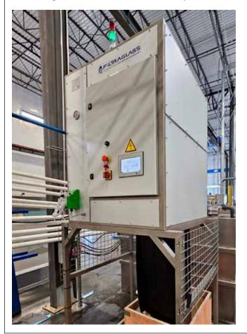
With the deployment of its DG.365 model at Elevation Glass in Denver, Colorado, FILTRAGLASS marks a significant success story for a system that allows for continuous operation without halting production, boosting productivity while recycling water and converting glass dust into recyclable waste - all in alignment with current environmental sustainability goals.
