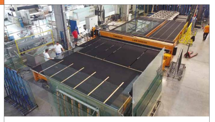
process in the cutting of jumbo laminated glass panels - making it possible to maximise all resources to achieve high quality results, even in large thicknesses. These machines feature advanced control technology - offering remarkable speed and pre-
