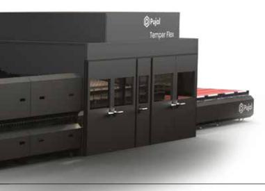
coating that helps to uniformly transmit the heat on the rollers and glass - a solution with lower energy consumption and greater speed and energy efficiency than traditional systems that protect inferior resistances based upon metal sheets on the screed. In the long run this offers lower energy consumption and lower maintenance costs - both in terms of sheet replacement and cleaning maintenance times when
