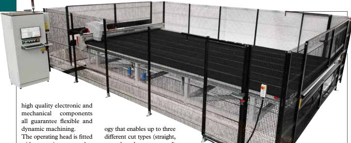
with an optic scanner that automatically detects the positioning of the sheet on the work table, which has a felt cover with integrated belts (retractable thanks to a 2-way drive). Precise, highquality cuts are achieved by controlling the pressure with a proportional valve connected to a display on the head. The optic scanner automatically detects the position of the sheet without operator intervention, thereby increasing both efficiency and productivity.
