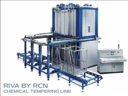
glass -from a minimum of 0.5 mm- can now lighten certain final installations without compromising safety. Despite the relatively long process time the benefits remain very significant as compared to other hardening solutions. After the lamination process, chemicallytempered glass becomes high-safety glass. Being very strong, chemically-tempered glass that's laminated is difficult to break. It will also stand in place before collapsing offering time enough for people to repair to safety.
