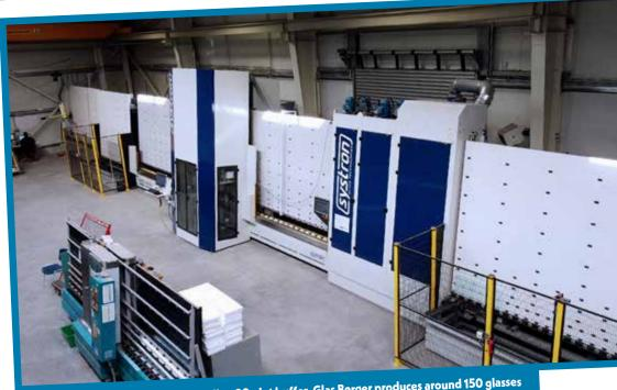
With the systron 3525proHD including 20-slot buffer, Glas Berger produces around 150 glasses with a wide variety of shapes and cut-outs per shift.
