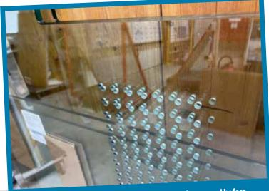
The systron waterjet cut holes do not need to be seamed before the tempering process.
